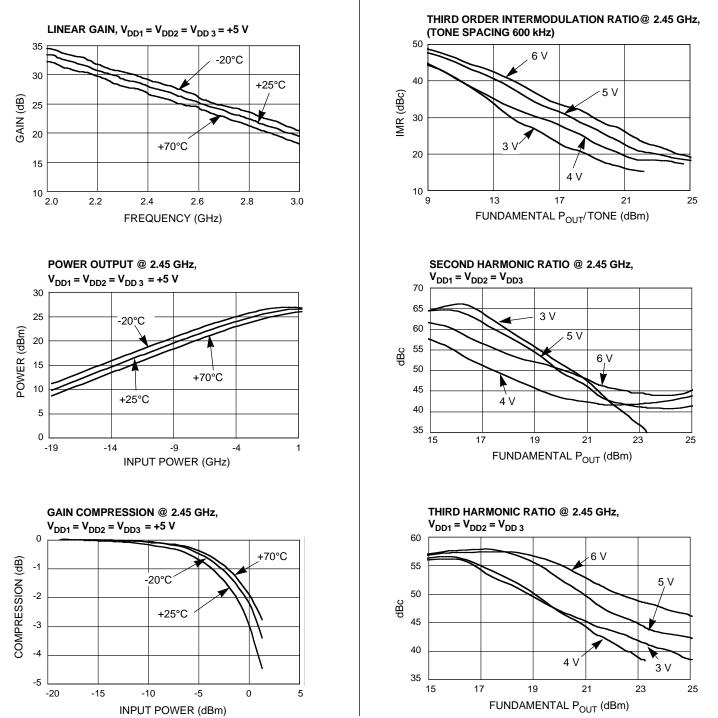
1. All data measured at T<sub>A</sub> = +25°C and V<sub>G1</sub>, V<sub>G2</sub> and V<sub>G3</sub> adjusted for first stage quiescent current of 20 mA, second stage current of 70 mA and third stage current of 90 mA, respectively.
